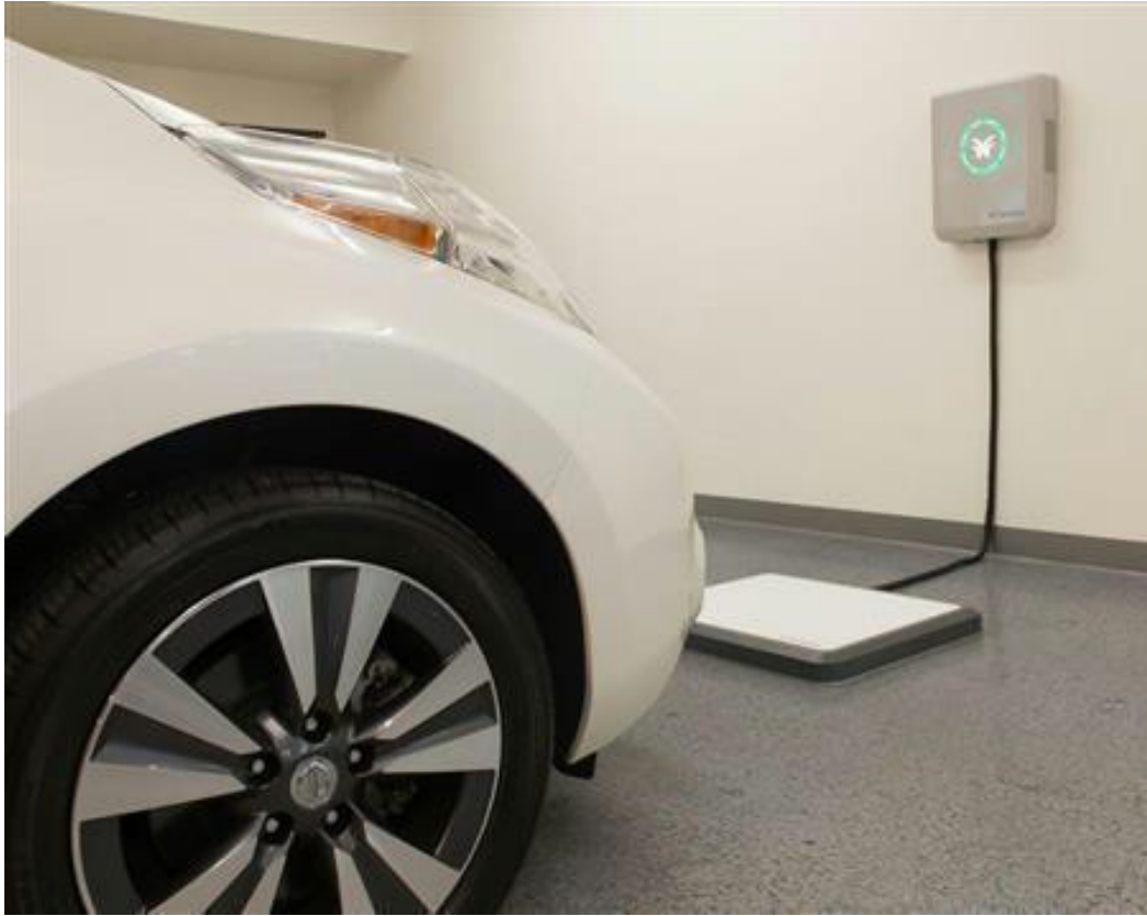
Figure 1. Wireless power transfer system of an EV and PHEV.
