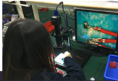
Wire terminal checking
